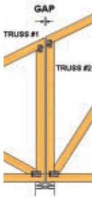
Two trusses sharing a wall
